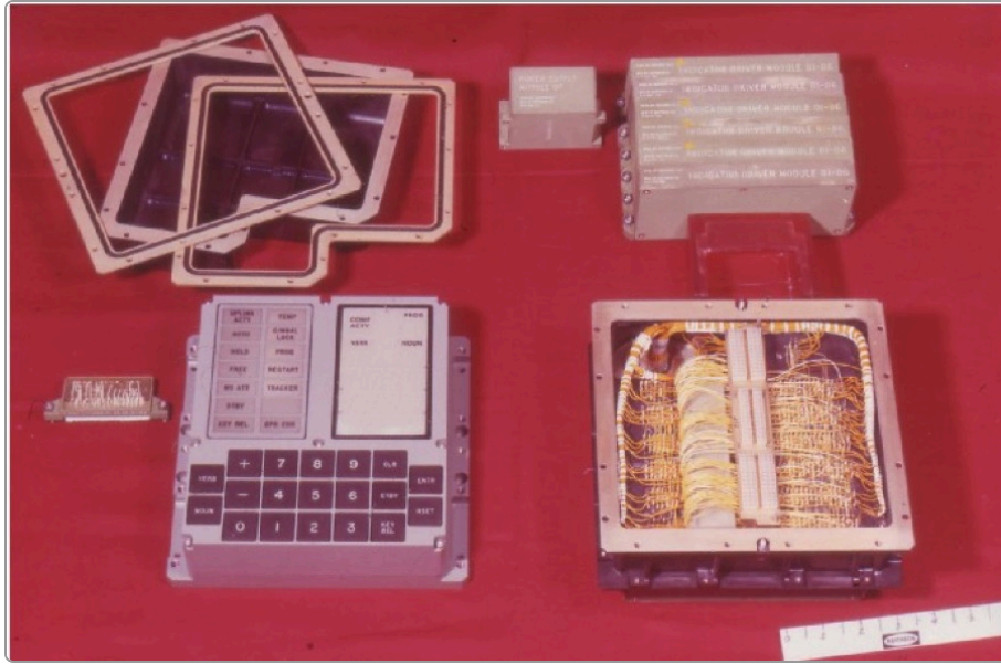
The Apollo Guidance Computer's Display and Keyboard, NASA, 1960s · Photograph · NASA
