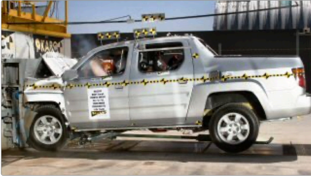
A Frontal Crash Test , National Highway Traffic Safety Administration, 2006 · Photograph · U.S. Department of Transportation
