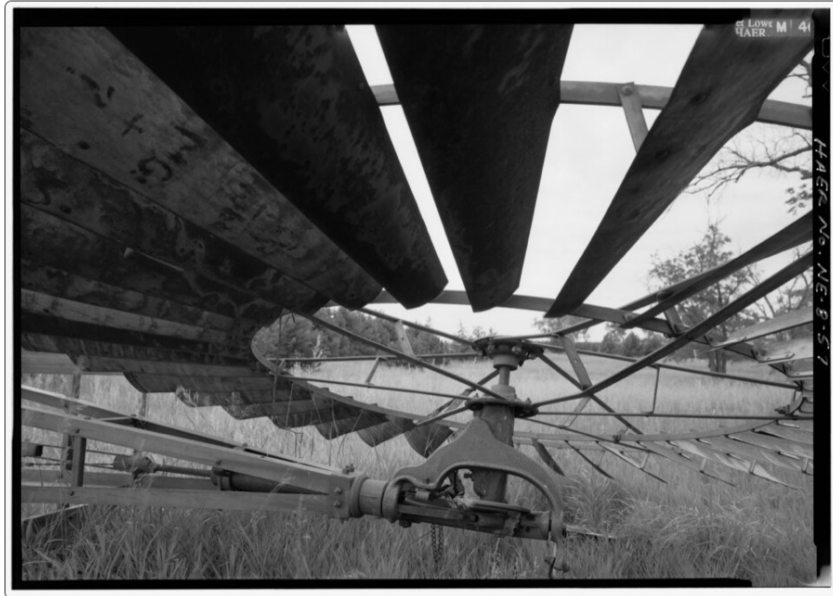
The Head and Wheel of a Water-Pumping Windmill , Historic American Engineering Record, survey photograph · Photograph · Kregel Windmill Company records, Nebraska City; Library of Congress
