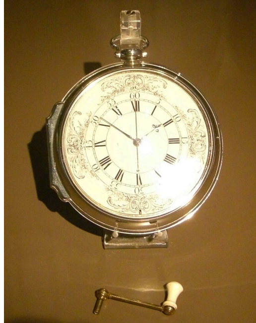
H4 Marine Timekeeper, John Harrison, 1759 · Silver case, with a movement of brass and steel and jeweled bearings · Royal Observatory, Greenwich (Royal Museums Greenwich)
