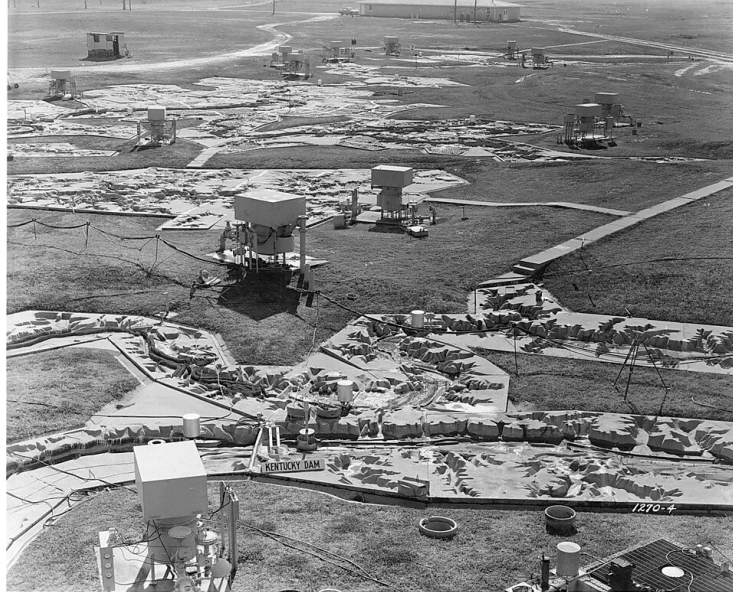
Mississippi Basin Model Vertical scale - 1:100; horizontal scale - 1:2000. Looking upstream on the Ohio River from Evansville. Indiana, Tennessee, and Cumberland Rivers are in the foreground showing the site of the Kentucky and Barkley Dams. Tradewater and Green Rivers are shown center. File No. 1270-4
