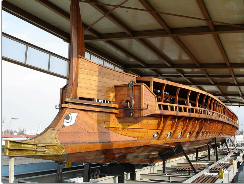
The Trireme Olympias , Built by the Hellenic Navy and the Trireme Trust; photograph by Templar52, Launched 1987 · Full-size working reconstruction of an Athenian trireme, in oak and pine · Naval Tradition Park, Palaio Faliro, near Athens
